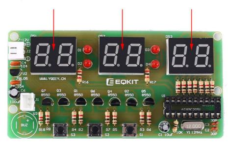
Step 18:Install 1pcs Active Buzzer at U3. Pay attention to the installation direction.
